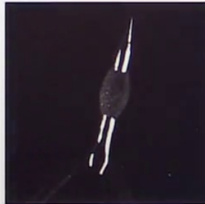
Schottky FEG with ZrO 2 reservoir and tip close-up
